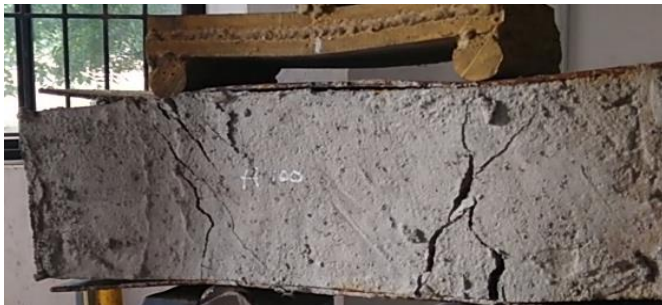
Figure 11 : Failure of the headed stud beam
