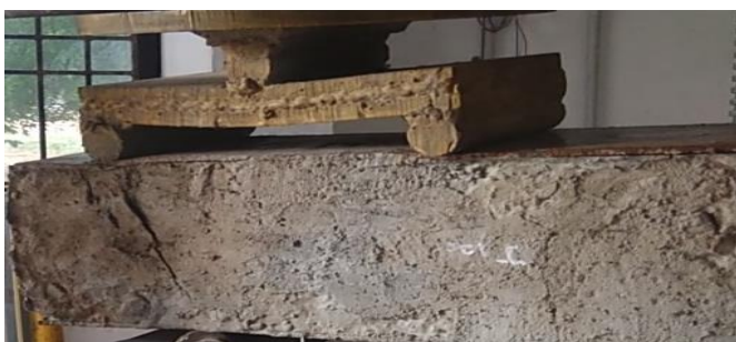
Figure 12: Failure of the J hook beam
