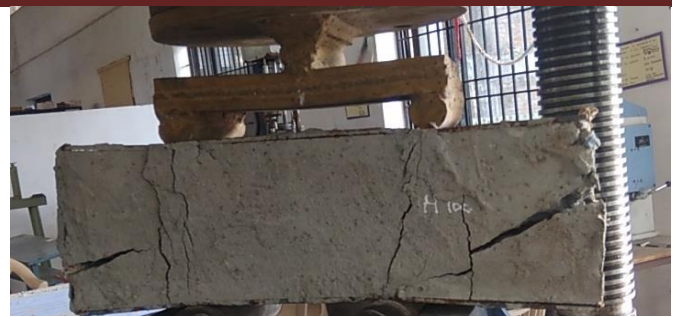
Figure 13 :Shear failure of the beam at ultimate stage
