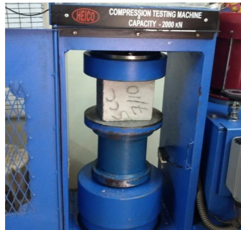
Figure 8 :Compressive tests for cube
