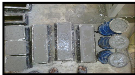
Figure 3: Casting of selfcuring concrete specimen
